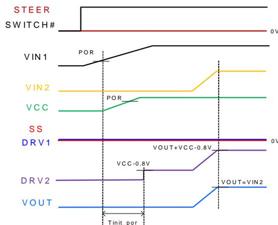
Figure 4. Power-Up Sequence of Scenario 2
