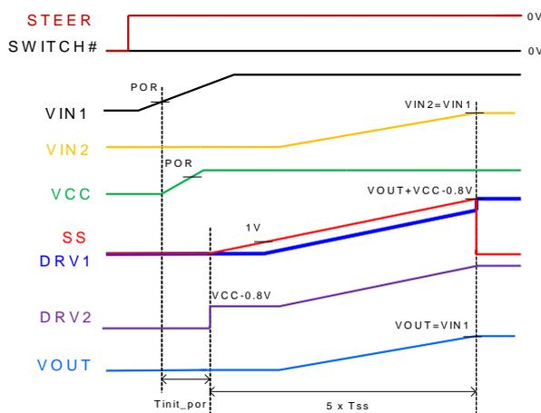
Figure 5. Power-Up Sequence of Scenario 3
