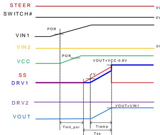
Figure 3. Power-Up Sequence of Scenario 1
