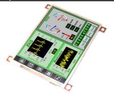
The uLCD-32PT(GFX) is a compact and cost effective all in one 'SMART" display module using the latest state of the art LCD (TFT) technology with an embedded PICASO-GFX2 graphics controller that delivers 'stand-alone' functionality to any project.
