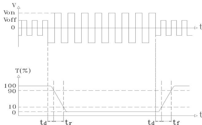
Turn on time:  $t_{on} = t_d + t_r$       Turn off time:  $t_{off} = t_d + t_f$
