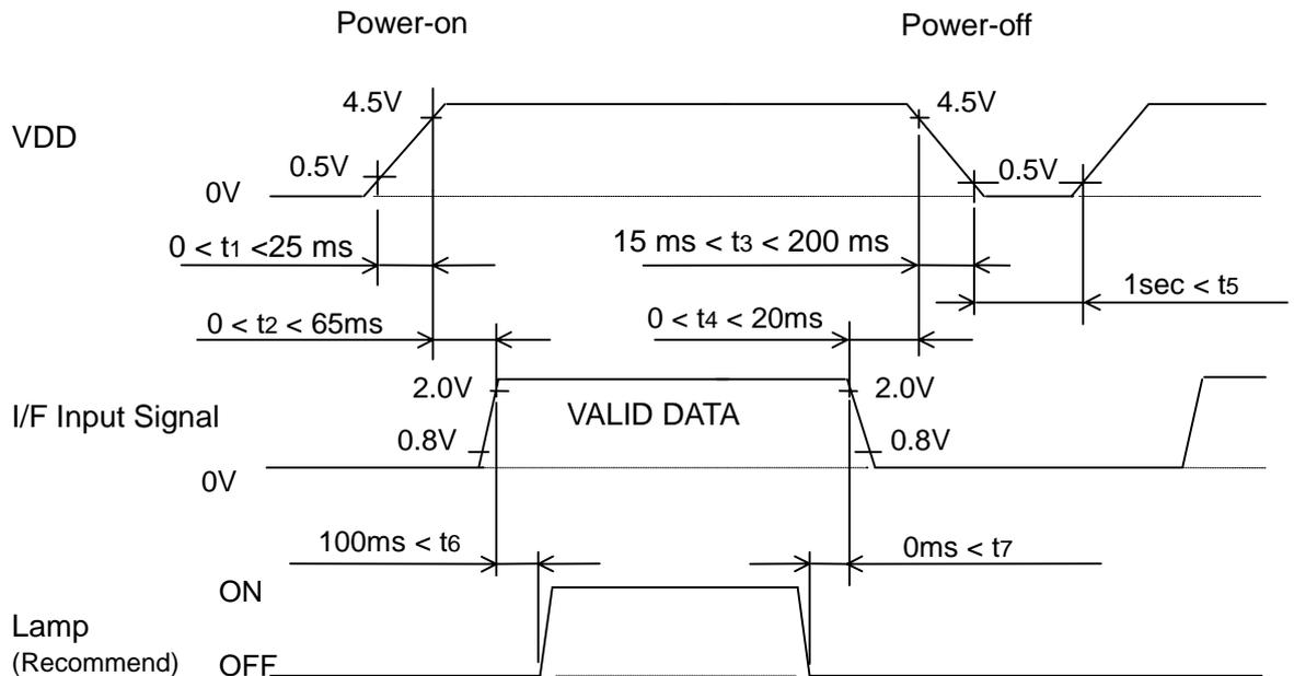
When the power is off, I/F Input Signal must be kept at either low level or high impedance.
