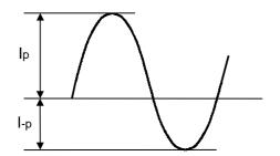
Unbalance rate =  $| I_p - I_{-p} | / I_L \times 100$  (%) Wave-height rate =  $I_p$  (or  $I_{-p}$ ) /  $I_L$
