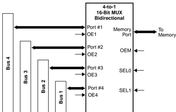
Note: All OE and SEL lines driven by external arbiter logic (not shown).
