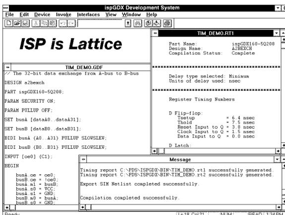
Status Bar and the work area. The figure below shows these elements of the ispGDX GUI.
