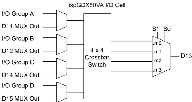
It can be seen from Figure 3 that if the D11 adjacent I/O cell is used, the I/O group “A” input is no longer available as a direct MUX input.
