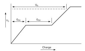
Basic gate charge waveform
