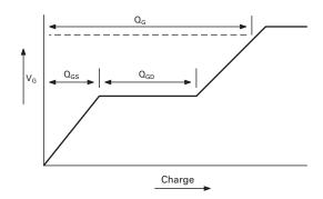
Basic gate charge waveform
