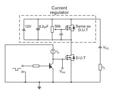
Gate charge test circuit
