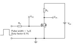
Switching time test circuit
