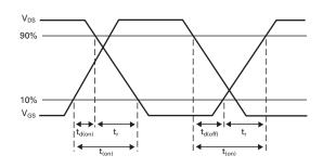
Switching time waveforms
