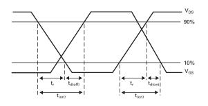
Switching time waveforms
