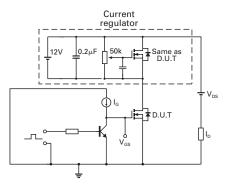
Gate charge test circuit
