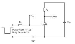
Switching time test circuit
