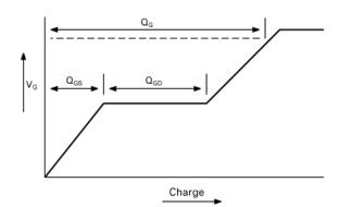
Basic gate charge waveform
