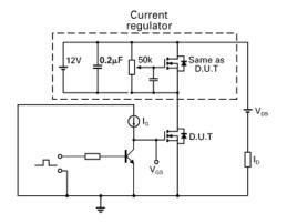
Gate charge test circuit
