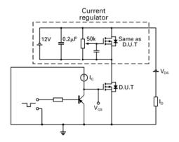
Gate charge test circuit
