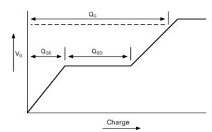
Basic gate charge waveform
