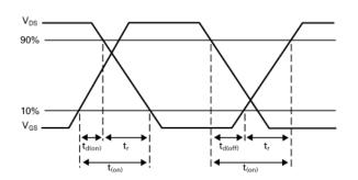
Switching time waveforms
