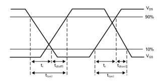
Switching time waveforms
