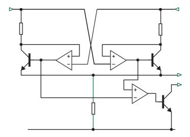
A common application for micro-power current monitors is measuring the discharge current of a rechargeable lithium ion/polymer battery. The ZXCT1041 enables measuring both the charge and discharge current into the battery and with its wide operating voltage of 2.5 to 20V enables it to measure the currents in to/ out of up to 4 cells connected in series.
