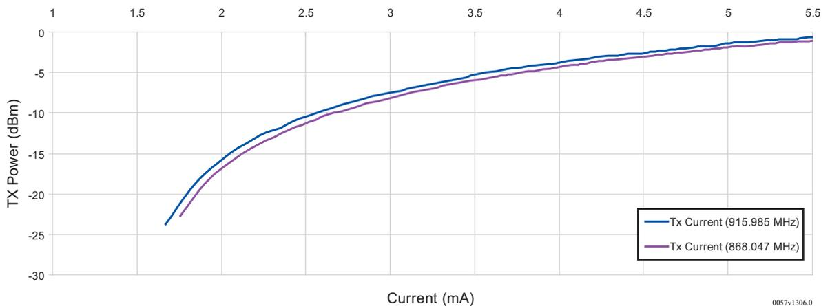
Figure 3-2 • TX Power vs. Current Consumption
