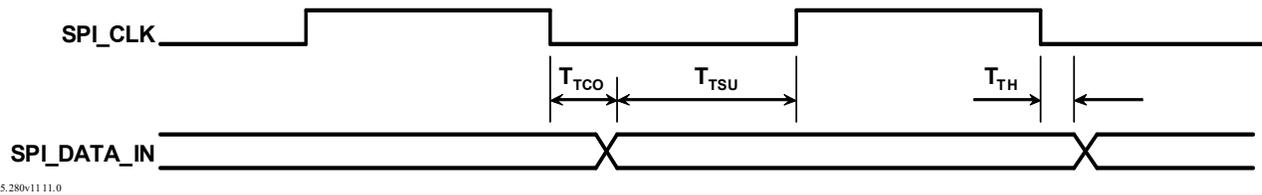
**Figure 2-3 • SPI Transmit Timing, External Microcontroller to ZL70251**
