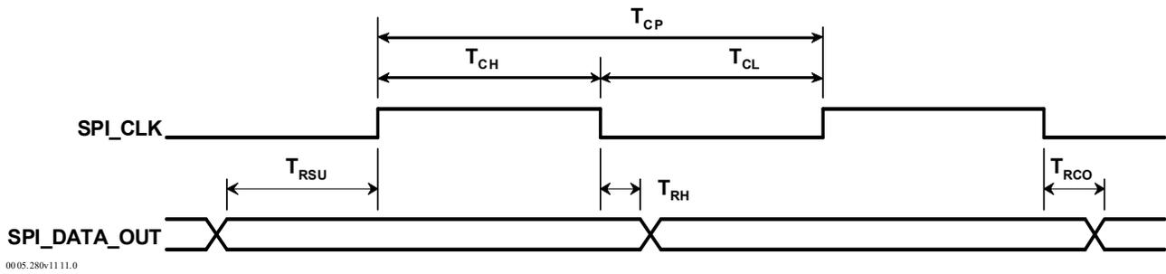
**Figure 2-2 • SPI Receive Timing, ZL70251 to External Microcontroller**
