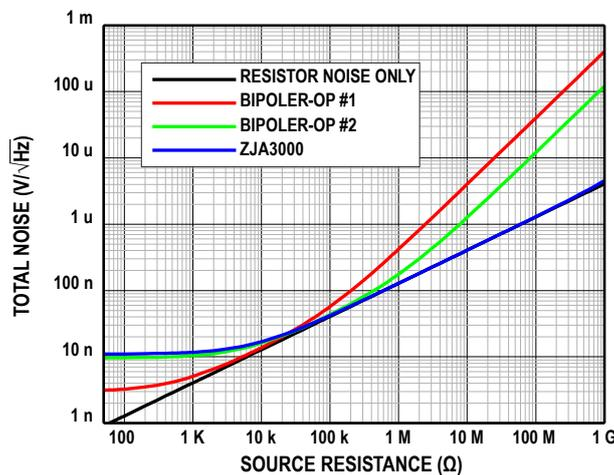
Figure 37. System Total Noise vs. Source Impedance
