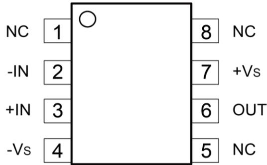
Figure 1. ZJA3000-1 Pin Configuration (8-lead SOIC and MSOP)
