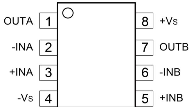
Figure 2. ZJA3000-2 Pin Configuration (8-lead SOIC and MSOP)
