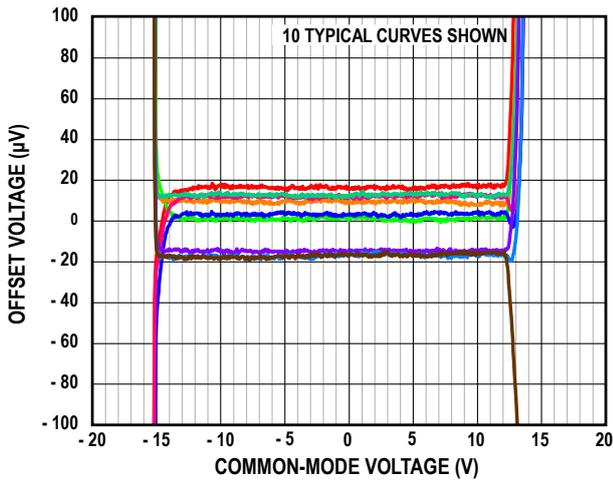
Figure 10. Offset Voltage vs. Input Common-Mode Voltage
