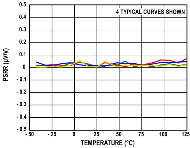
Figure 22. Power Supply Rejection Ratio (PSRR) vs. Temperature
