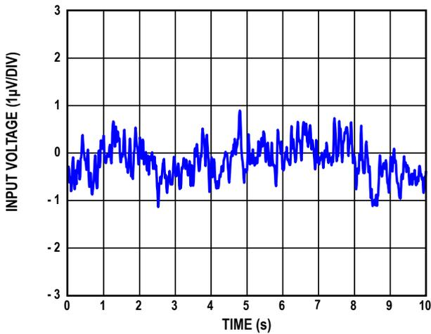
Figure 32. 0.1 Hz to 10 Hz Noise
