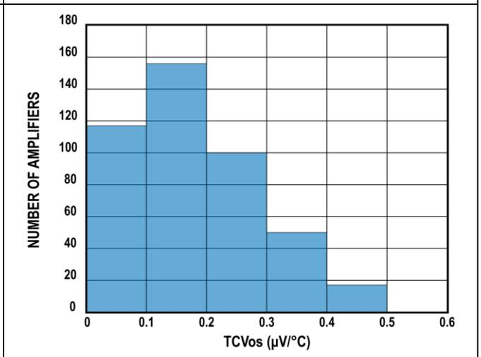
Figure 9. Input Offset Voltage Drift Distribution, SOIC-8 Package
