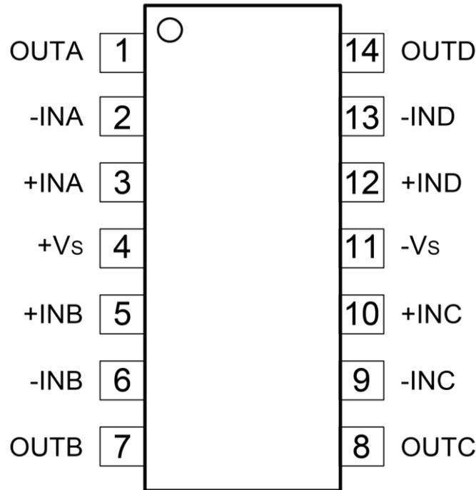
Figure 3. ZJA3000-4 Pin Configuration (14-lead SOIC and TSSOP)
