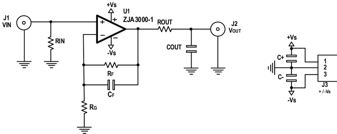
Figure 42. Op Amp Schematic for Non-inverting Configuration
