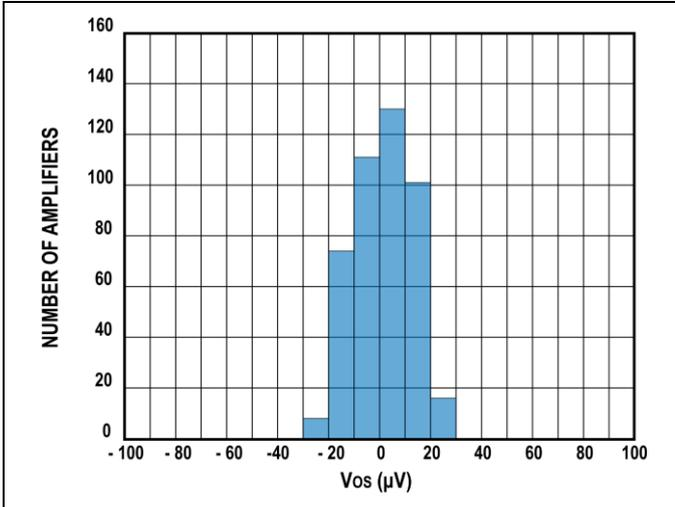
Figure 4. Input Offset Voltage Distribution, SOIC-8 Package
