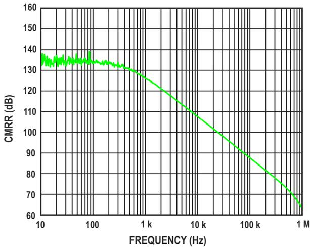
Figure 24. Common Mode Rejection Ratio (CMRR) vs. Frequency
