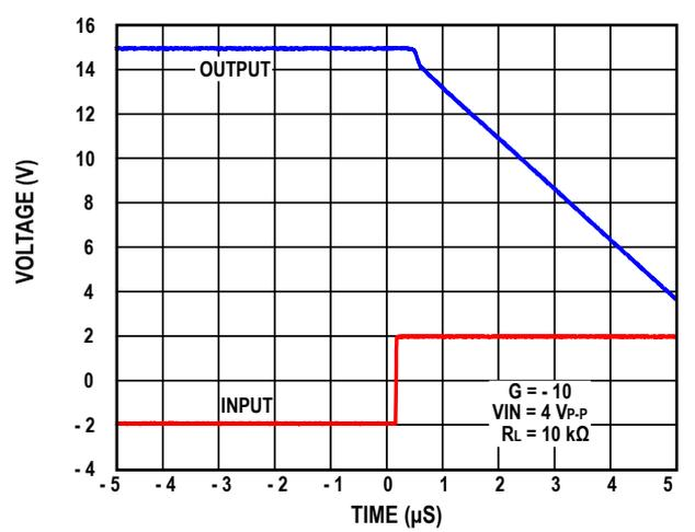
Figure 21. Negative Overload Recovery
