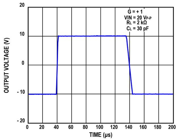
Figure 19. Large Signal Transient Response
