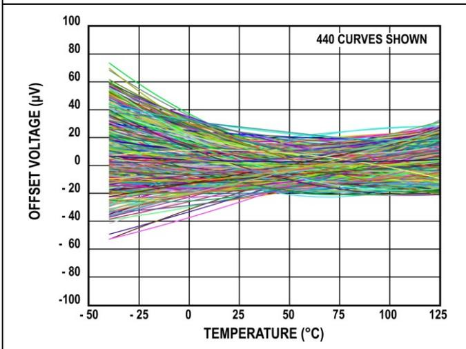
Figure 8. Input Offset Voltage vs. Temperature, SOIC-8 Package
