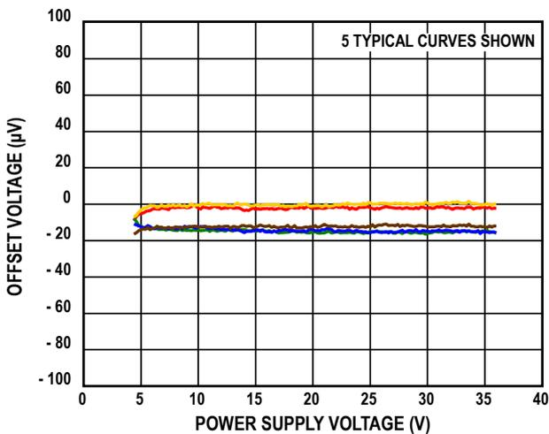
Figure 14. Input Offset Voltage vs. Power Supply Voltage
