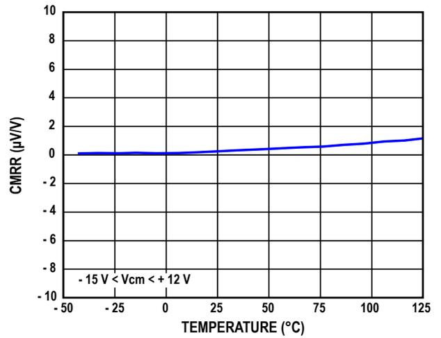
Figure 17. Common Mode Rejection Ratio (CMRR) vs. Temperature
