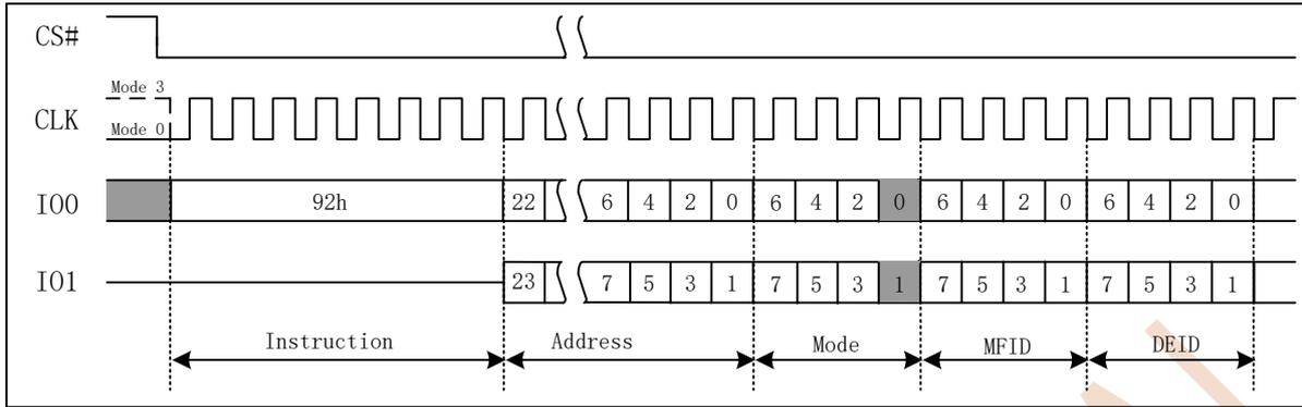
Figure 7.29 Read Manufacturer/Device ID Dual I/O Instruction
