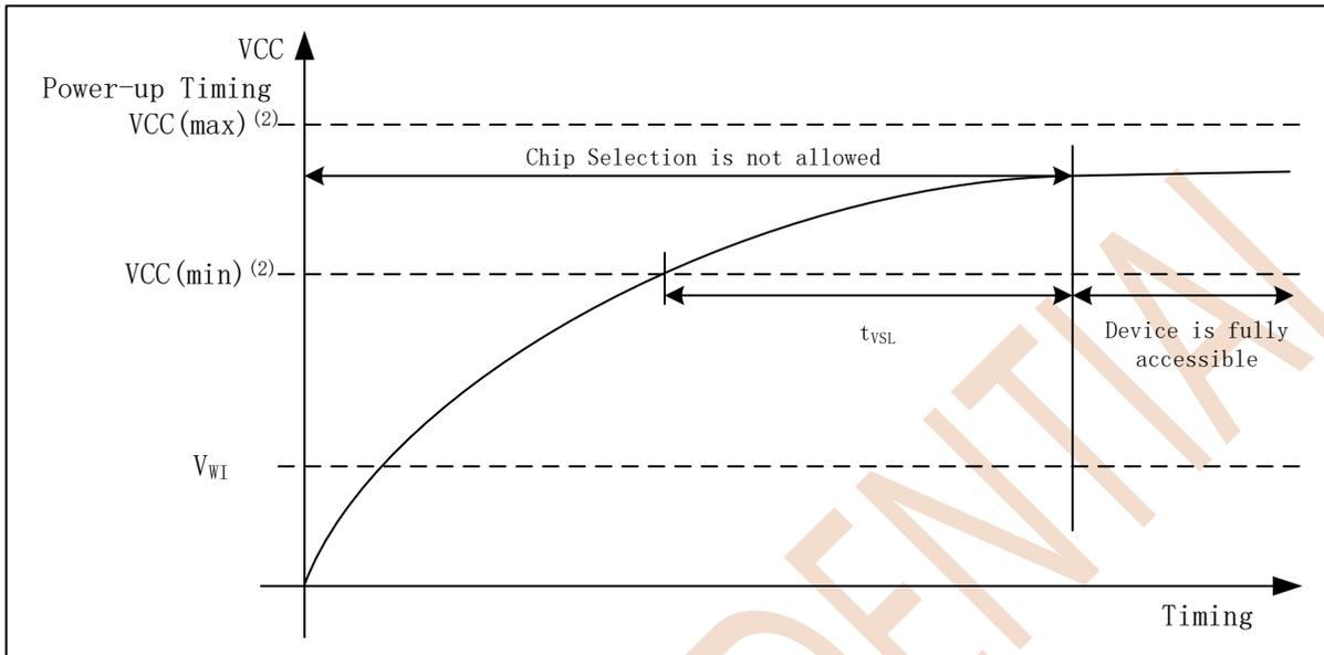
Figure 8.1 Power-up Timing
