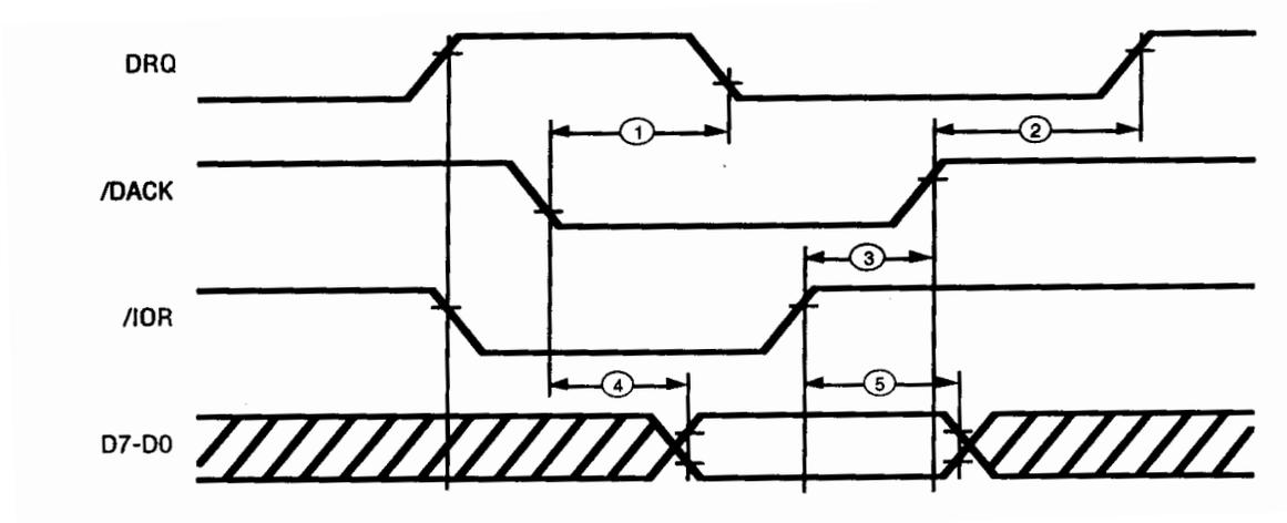
Figure 4. DMA Read Timing Diagram
