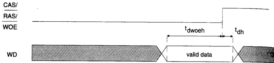
Figure 6. Sample Memory Read Timing Diagram
