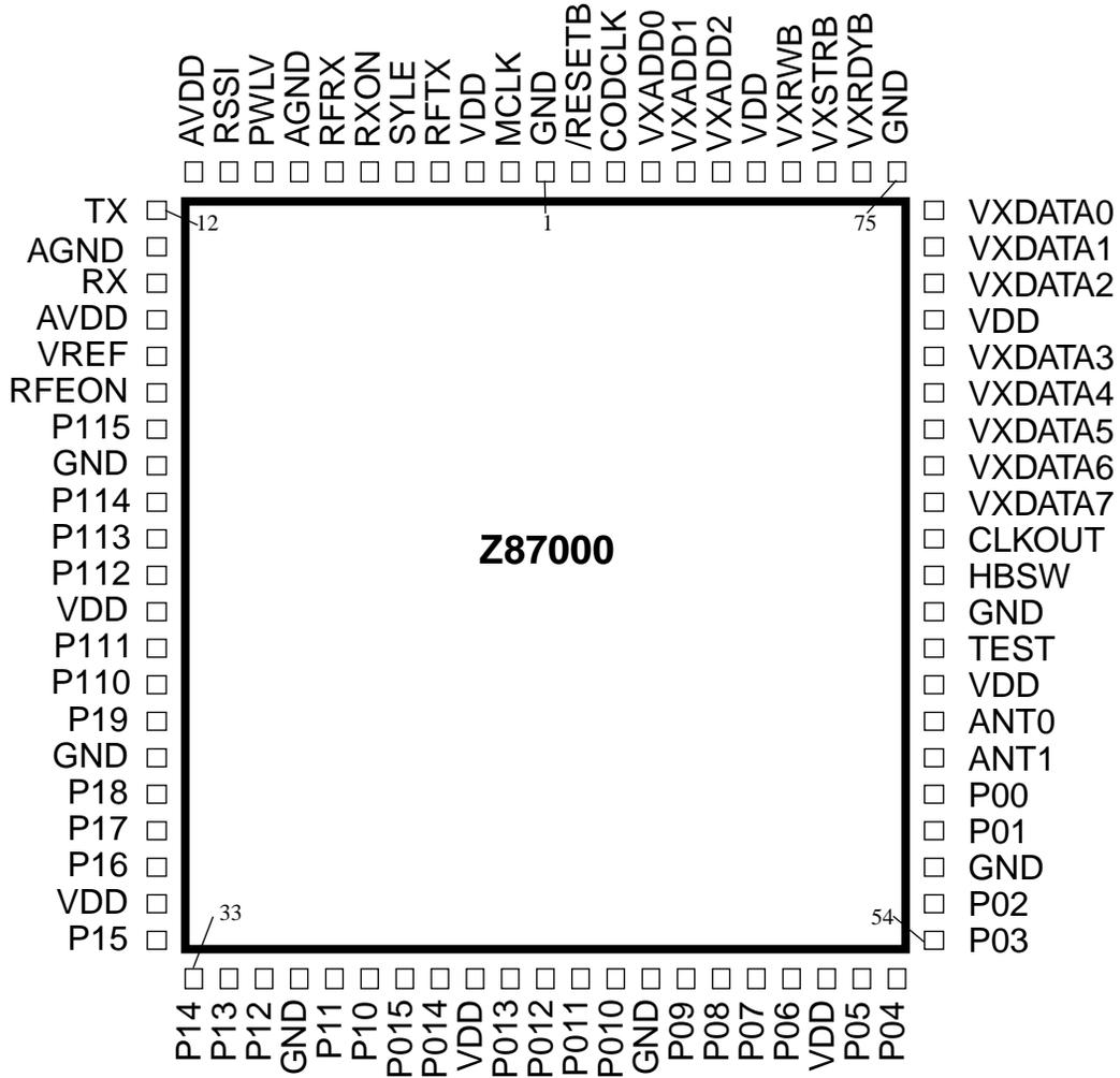
**Figure 3. 84-Pin PLCC ROM Pin Configuration (Z87000 only)**
