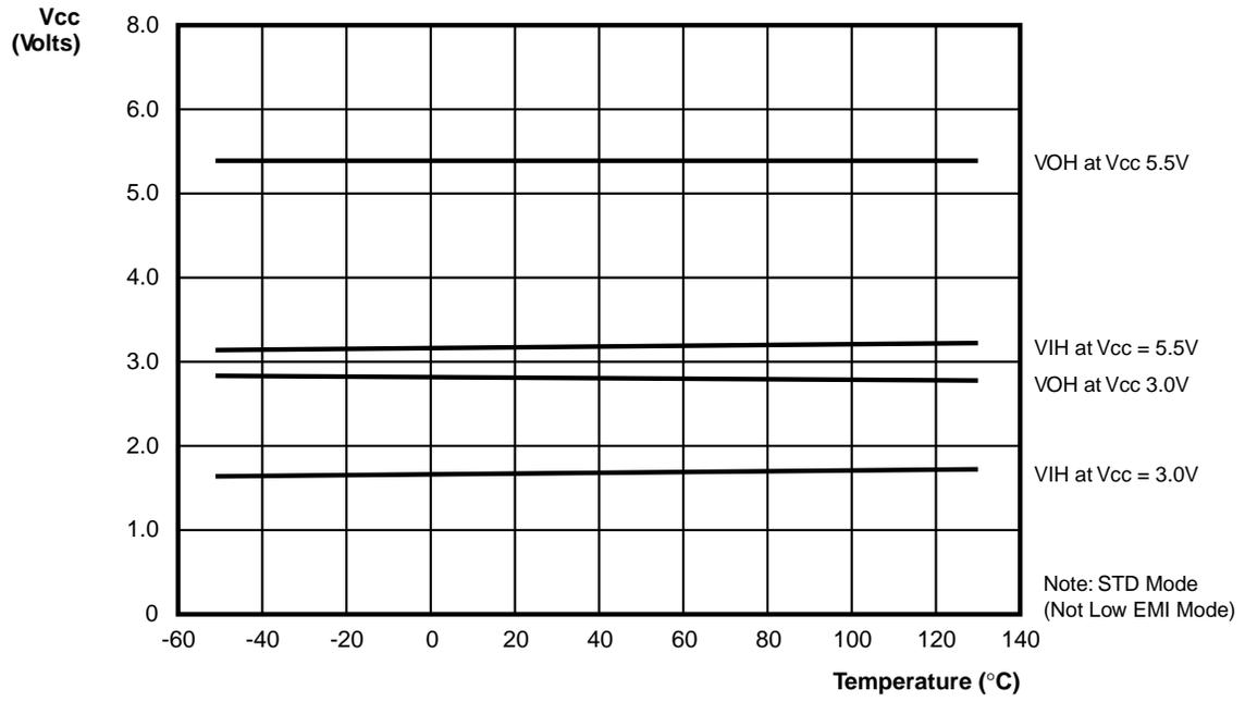
Figure 54. Typical V<sub>OH</sub>, V<sub>IH</sub> vs Temperature
