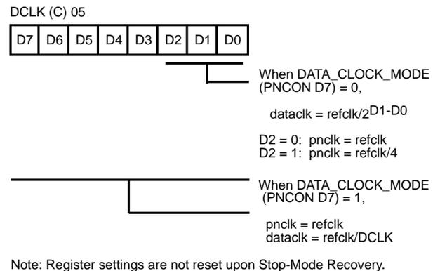
**Figure 40. Data Clock Control Register ((C) 05H: Read/Write)**
