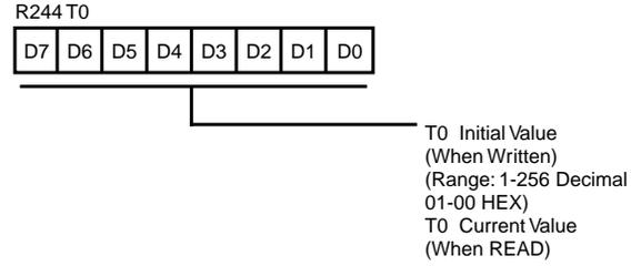
Figure 31. Counter Timer 1 Register (F2H: Read/Write)
