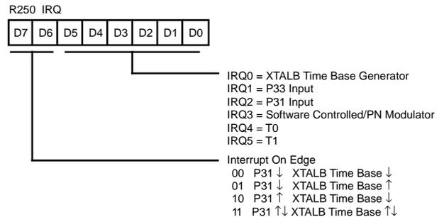
**Figure 46. Interrupt Request Register (FAH: Read/Write)**
