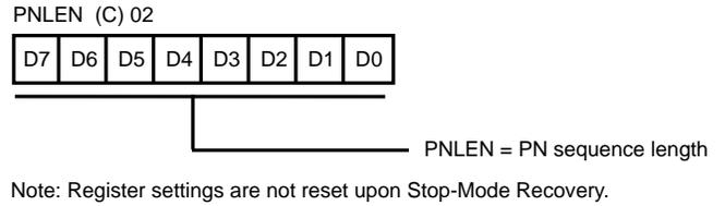
**Figure 37. PN Code Length Register ((C) 02H: Read/Write)**
