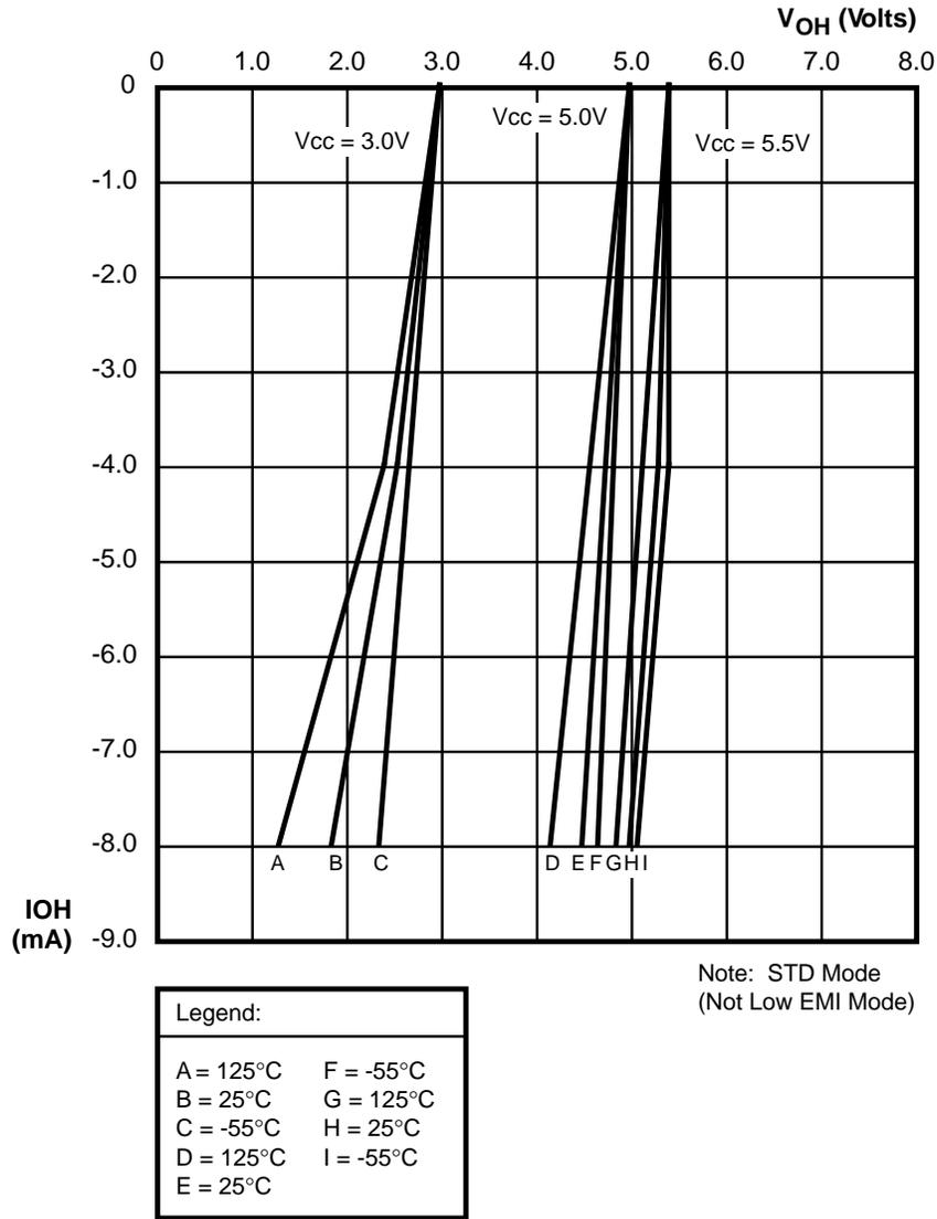
Figure 55. Typical V<sub>OH</sub> vs I<sub>OH</sub> Over Temperature
