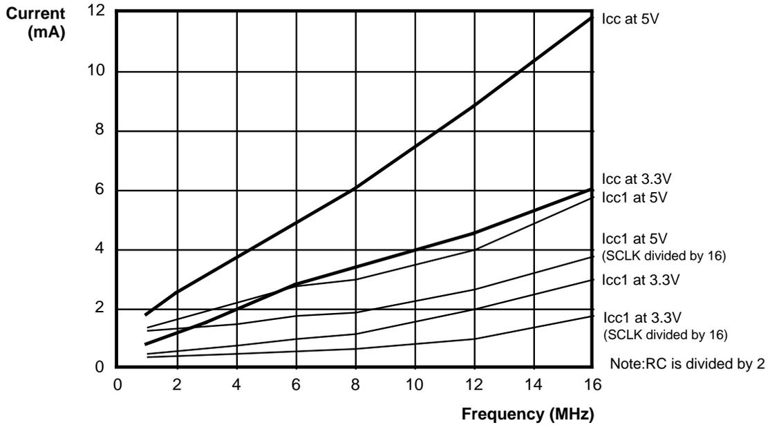
Figure 52. Typical I<sub>CC</sub> vs Frequency
