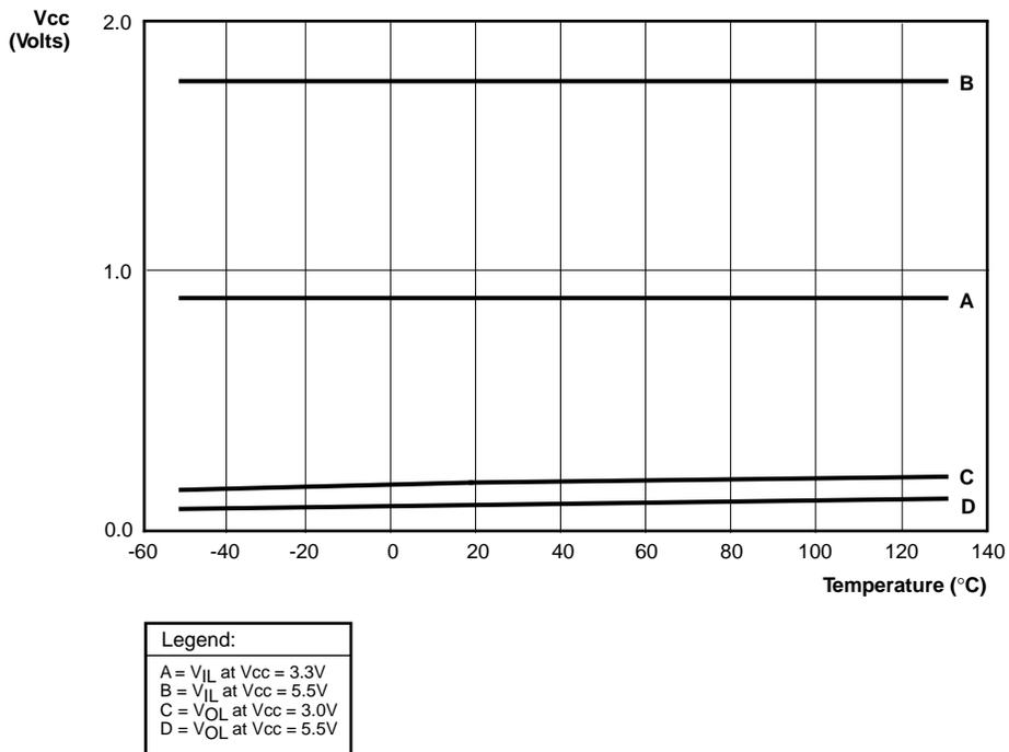
Figure 53. Typical V<sub>OL</sub>, V<sub>IL</sub> vs Temperature
