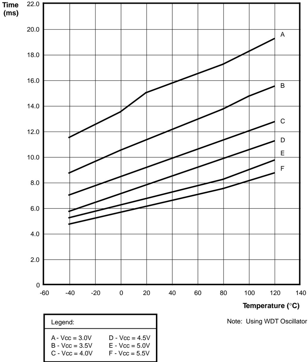
Figure 57. Typical Power-On Reset Time vs Temperature
