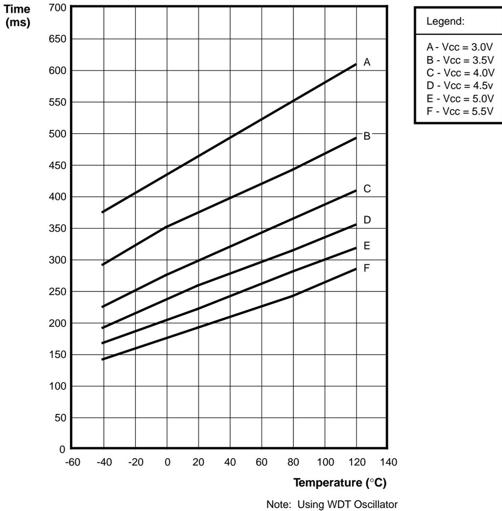
Figure 61. Typical 100 ms WDT Setting vs Temperature
