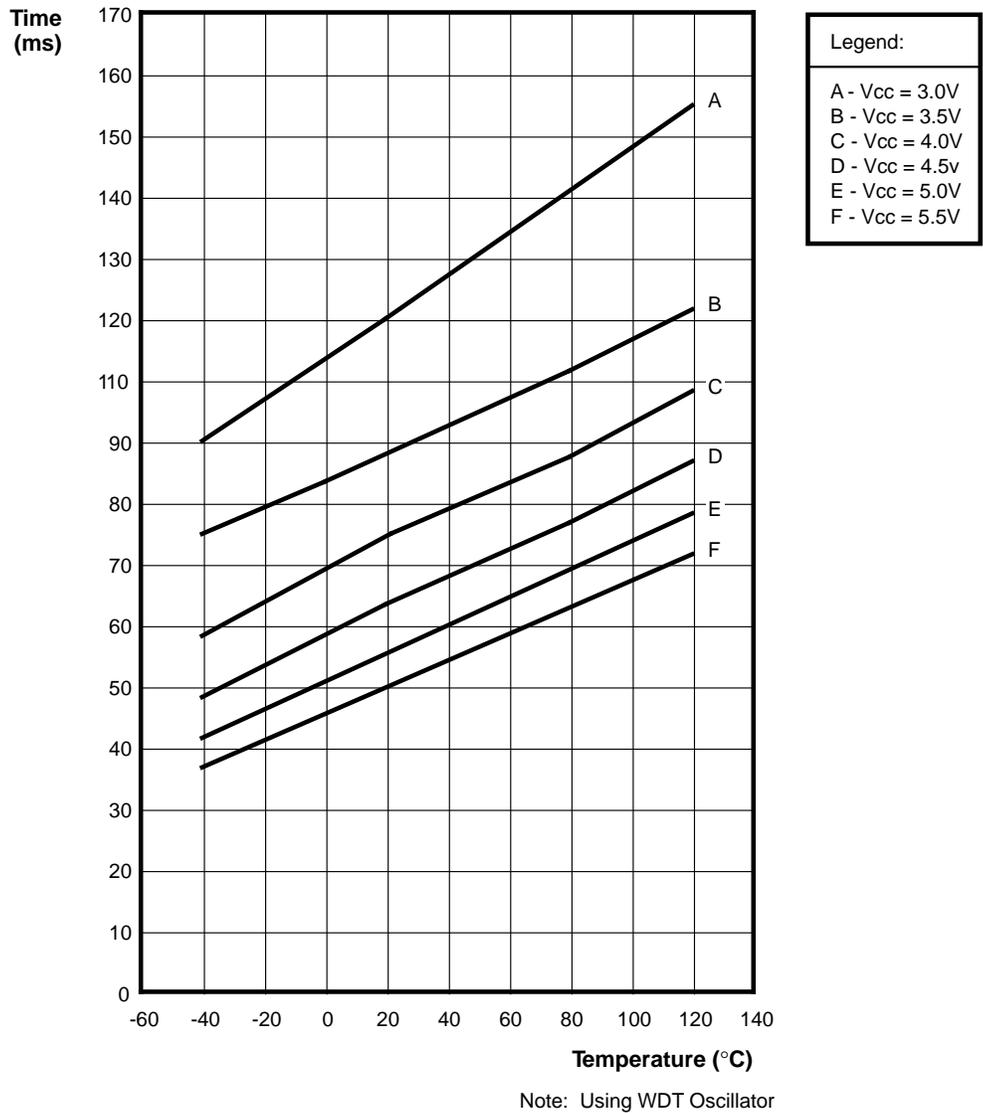
Figure 60. Typical 25 ms WDT Setting vs Temperature
