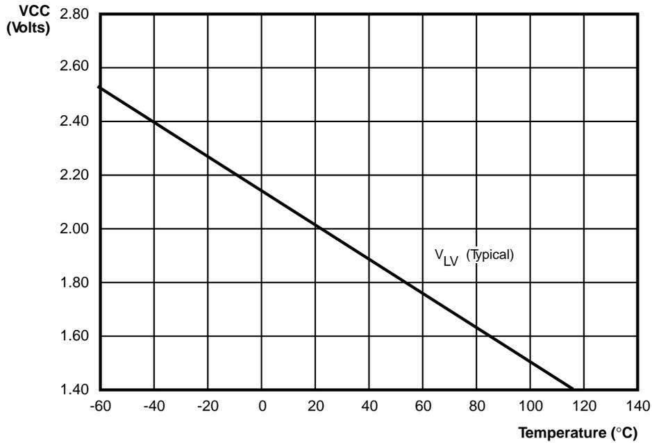
Figure 25. Typical Z87100 V<sub>LV</sub> Voltage vs Temperature
