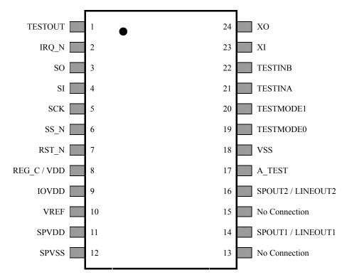
24-pin SSOP TOP View
