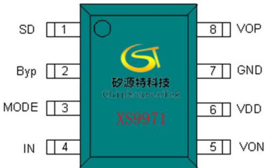
Figure 2 XS9971 Terminal definition
