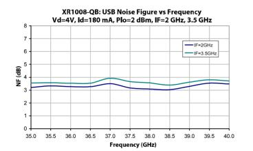
XR1008-QB: LSB Noise Figure vs Frequency Vd=4V, Id=180 mA, Plo=2 dBm, IF=2 GHz, 3.5 GHz 8 7 -IF=2GHz 6 IF=3.5GHz 5 (dB) Ľ 3 2 0 35.0 35.5 36.0 36.5 37.0 37.5 38.0 38.5 39.0 39.5 40.0 Frequency (GHz)
