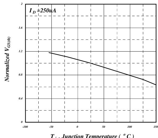
**Fig 6. Gate Threshold Voltage v.s. Junction Temperature**
