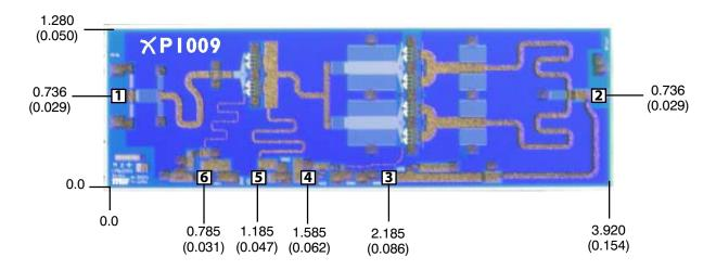
Units: millimeters (inches) Bond pad dimensions are shown to center of bond pad. Thickness: 0.110 +/- 0.010 (0.0043 +/- 0.0004), Backside is ground, Bond Pad/Backside Metallization: Gold All Bond Pads are  $0.100 \times 0.100 (0.004 \times 0.004)$ .
