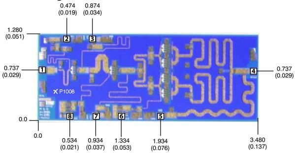
Units: millimeters (inches) Bond pad dimensions are shown to center of bond pad. Thickness: 0.110 +/- 0.010 (0.0043 +/- 0.0004), Backside is ground, Bond Pad/Backside Metallization: Gold All Bond Pads are  $0.100 \times 0.100 (0.004 \times 0.004)$ .
