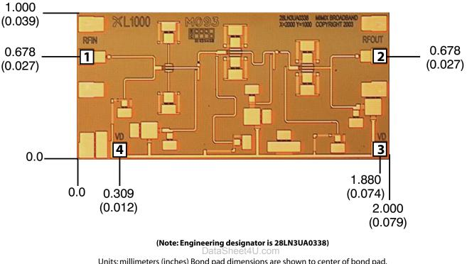
Units: millimeters (inches) Bond pad dimensions are shown to center of bond pad. Thickness: 0.110 +/- 0.010 (0.0043 +/- 0.0004), Backside is ground, Bond Pad/Backside Metallization: Gold All Bond Pads are 0.100 x 0.100 (0.004 x 0.004). Bond pad centers are approximately 0.109 (0.004) from the edge of the chip. Dicing tolerance: +/- 0.005 (+/- 0.0002). Approximate weight: 1.239 mg.
