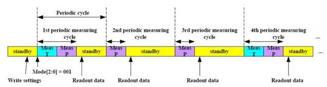
FIFO Mode: The XGZP6806 has a set of FIFO registers capable of storing 32 bridge sensor measurements. It helps to improve system power consumption. In FIFO mode, measurements are performed in a continuous loop until the FIFO register is filled with 32 measurements. Once the data is read and the FIFO register is not full, the measurement starts automatically until the data fills up again
