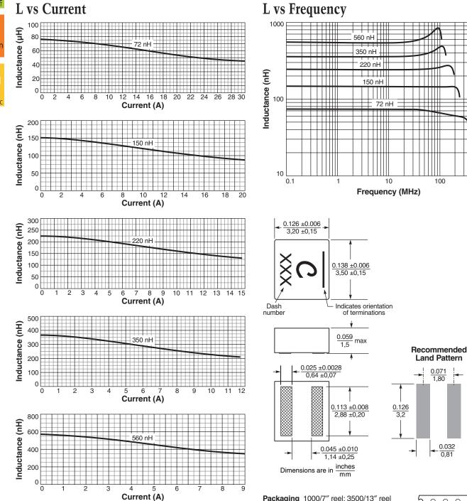
**Packaging** 1000/7" reel; 3500/13" reel Plastic tape: 12 mm wide, 0.23 mm thick, 8 mm pocket spacing, 1.8 mm pocket depth
