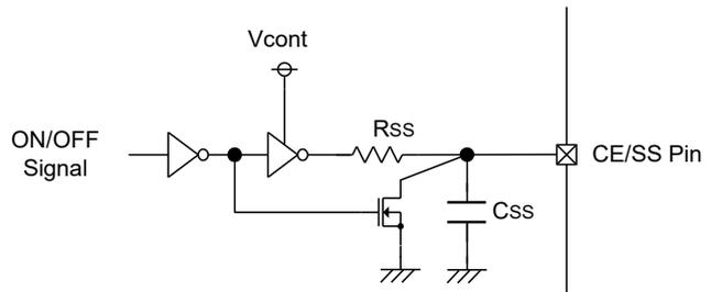
Ex.) Reference Circuit 2: CMOS Logic (Low Supply Current)
