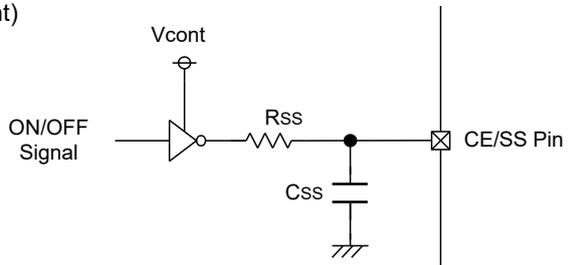
Ex.) Reference Circuit 3: CMOS Logic (Low Supply Current), Quick-Off
