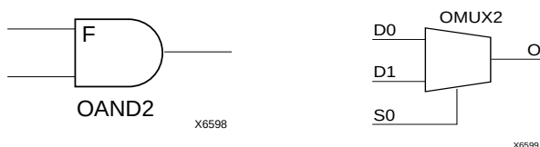
Figure 20: AND & MUX Symbols in XC4000X IOB
