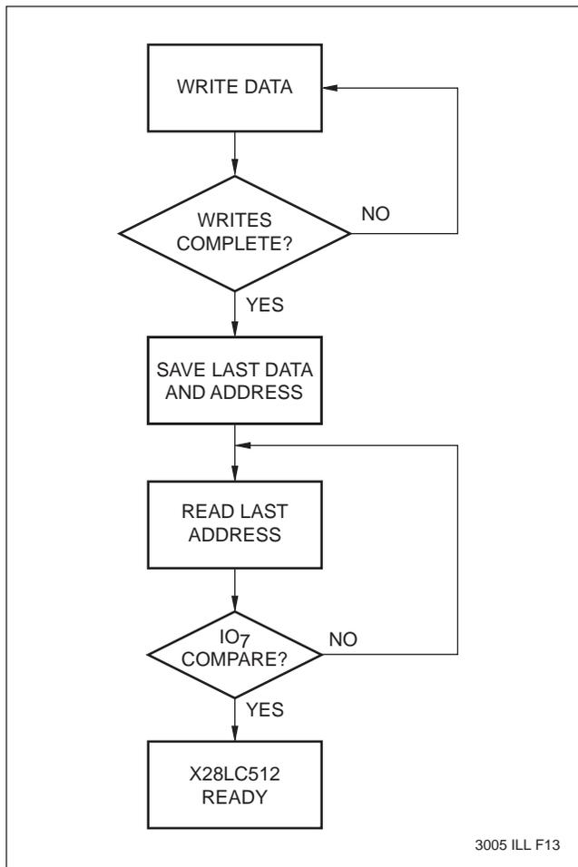
DATA Polling can effectively halve the time for writing to the X28LC512/513. The timing diagram in Figure 2a illustrates the sequence of events on the bus. The software flow diagram in Figure 2b illustrates one method of implementing the routine.
