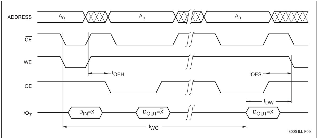
**Toggle Bit Timing Diagram**
