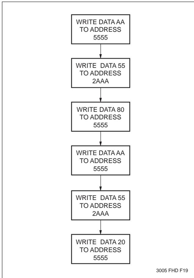
In the event the user wants to deactivate the software data protection feature for testing or reprogramming in an E<sup>2</sup>PROM programmer, the following six step algorithm will reset the internal protection circuit. After  $t_{WC}$ , the X28LC512/513 will be in standard operating mode.
