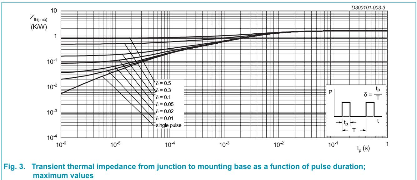
Fig. 3. Transient thermal impedance from junction to mounting base as a function of pulse duration; maximum values
