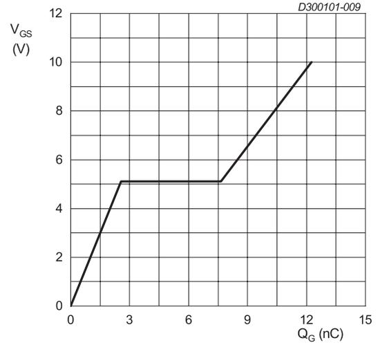
$I_D = 3.5 A; V_{DS} = 400 V$
