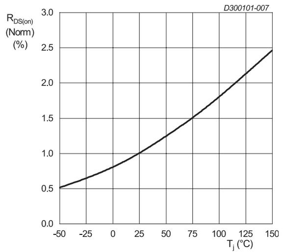
$V_{GS} = 10\text{ V}; I_D = 3.5\text{ A}$
