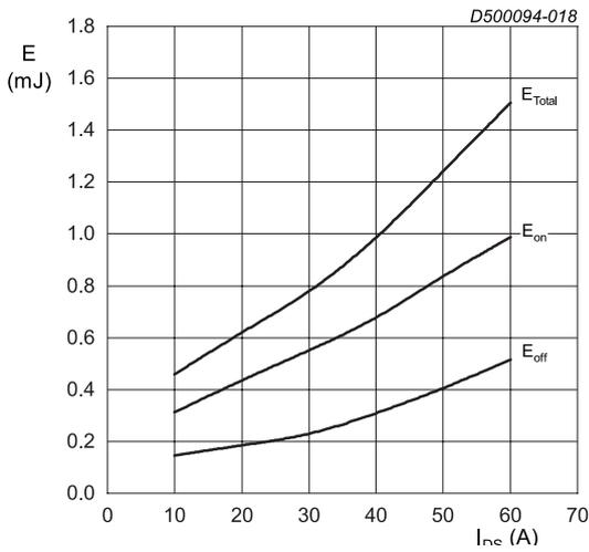
T<sub>j</sub> = 25 °C; V<sub>DD</sub> = 800 V; R<sub>G(ext)</sub> = 2.4 Ω; R<sub>G(on)</sub> = 2.4 Ω;
