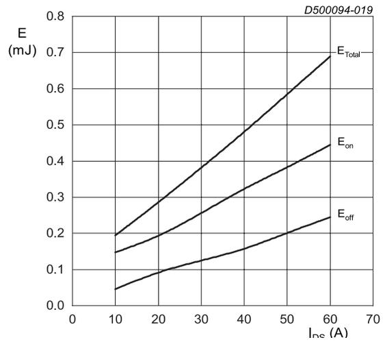
T<sub>j</sub> = 25 °C; V<sub>DD</sub> = 600 V; R<sub>G(off)</sub> = 2.4 Ω; R<sub>G(on)</sub> = 2.4 Ω;
