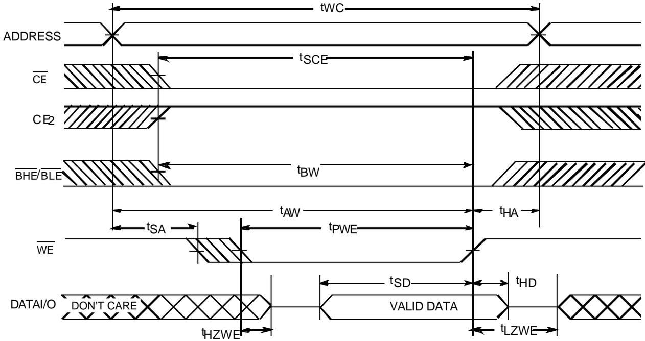
**Write Cycle No. 4 ( $\overline{BHE}/\overline{BLE}$  Controlled,  $\overline{OE}$  LOW)<sup>[17, 18]</sup>**
