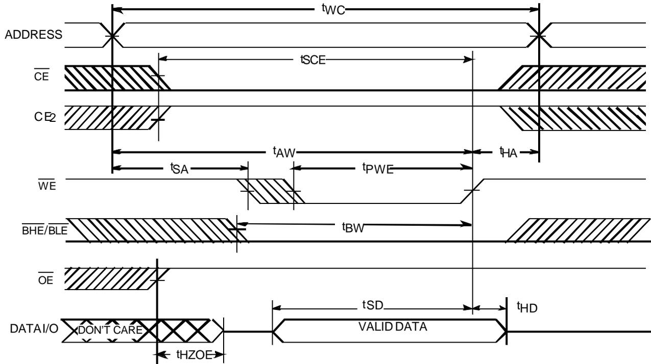
**Write Cycle No. 2 ( $\overline{CE}$  Controlled)**<sup>[13, 14, 16, 17, 18,]</sup>
