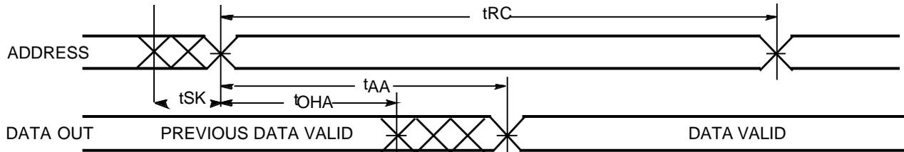
Read Cycle No. 2 ( $\overline{OE}$  Controlled) <sup>[15]</sup>
