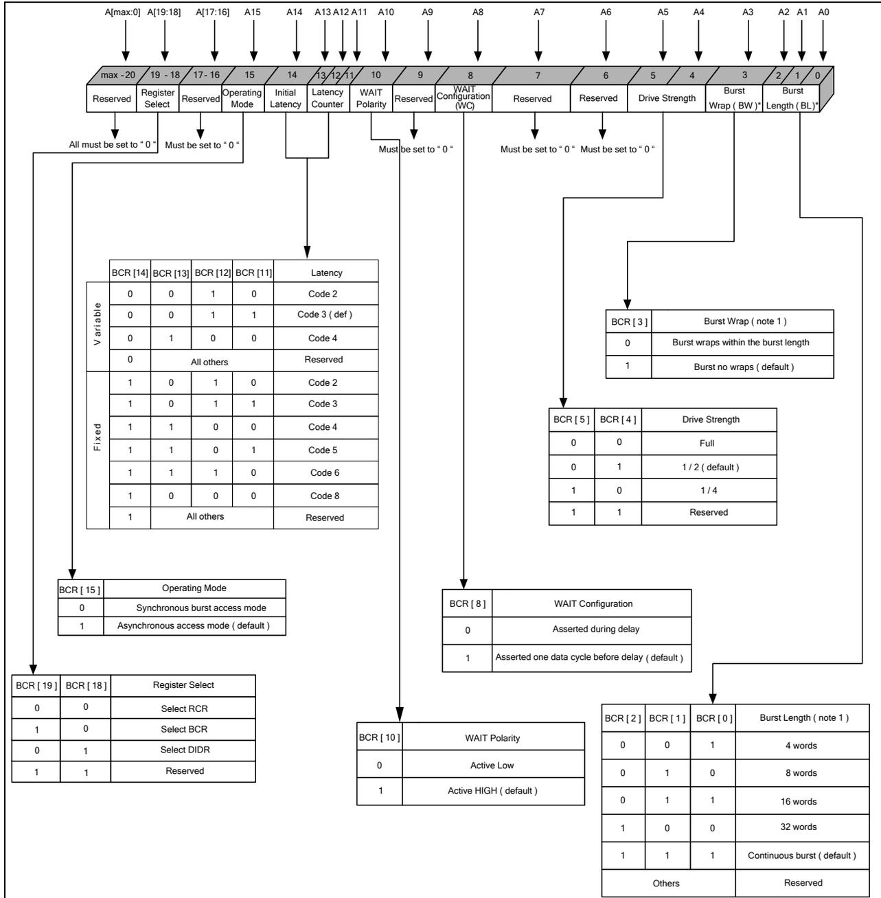
Note: 1. Burst wrap and length apply to both READ and WRITE operations.
