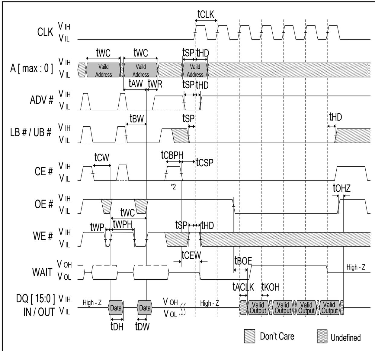
Note : 1. Non-default BCR settings for asynchronous WRITE ,with ADV# LOW, followed by burst READ: Fixed or variable latency; latency code 2(3 clocks); WAIT active LOW; WAIT asserted during delay.
