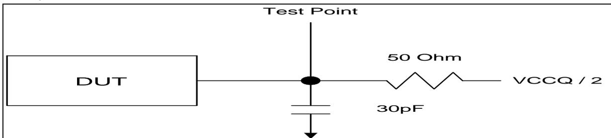
Note: All tests are performed with the outputs configured for default setting of half drive strength (BCR[5:4] = 01b).
