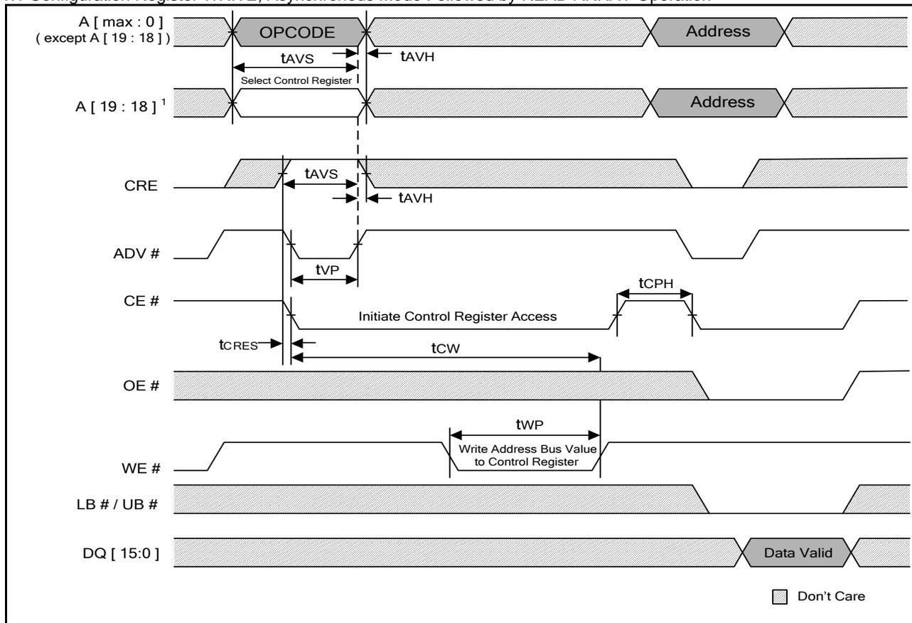
Note : 1. A[19:18]=00b to load RCR, and 10b to load BCR.
