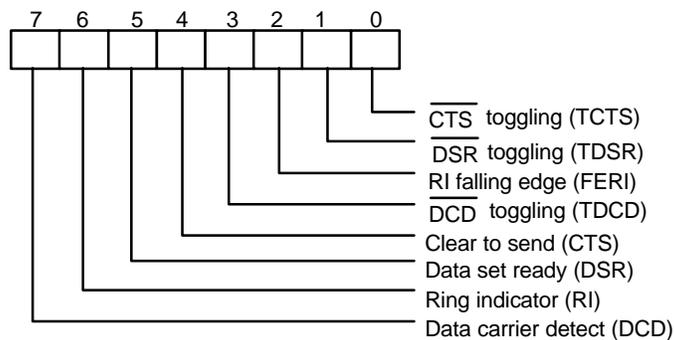
Bit 7: This bit is the opposite of the  $\overline{DCD}$  input. This bit is equivalent to bit 3 of HCR in loopback mode.
