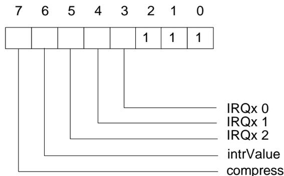
Bit 7: This bit is read-only. It is at low level during a read. This means that this chip does not support hardware RLE compression.
