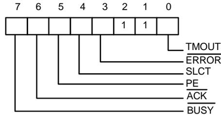
Bit 7: This signal is active during data entry, when the printer is off-line during printing, when the print head is changing position, or during an error state. When this signal is active, the printer is busy and cannot accept data.
