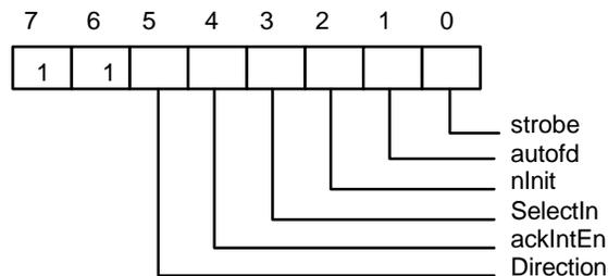
Bit 6, 7: These two bits are logic one during a read and cannot be written.
