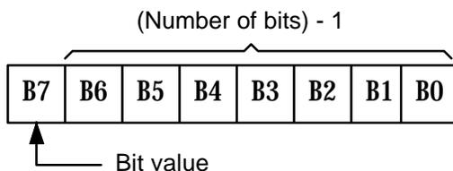
If the bit value is set to 0, the high pulse will be transmitted/received. If the bit value is set to 1, then no energy will be transmitted/received.
