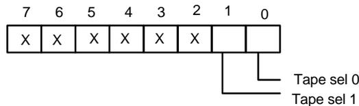
If three mode FDD function is enabled (EN3MODE = 1 in Logical Device 0 CRF0 bit:0), the bit definitions are as follows:
