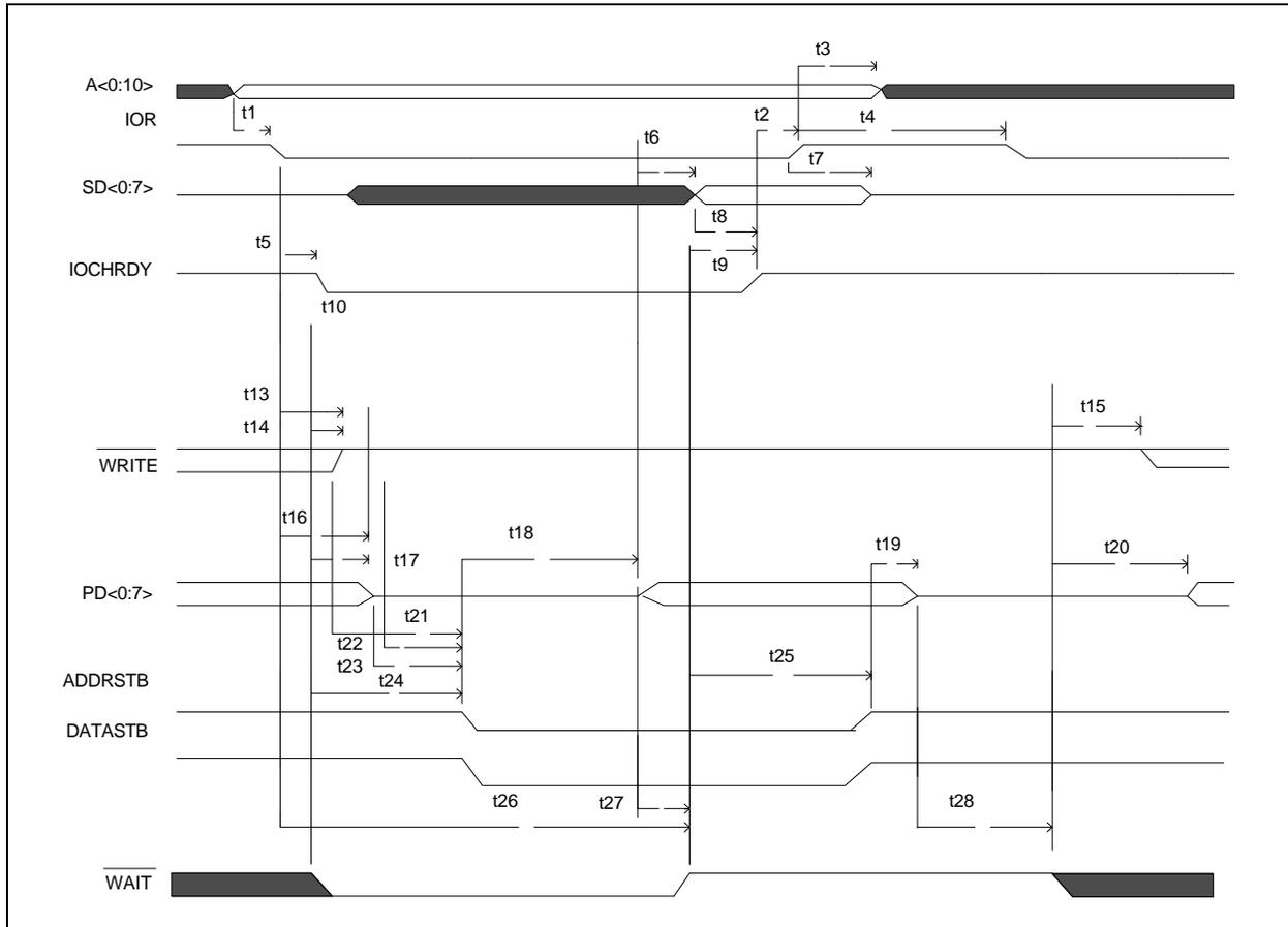
**12.3.5 EPP Data or Address Write Cycle (EPP Version 1.7)**
