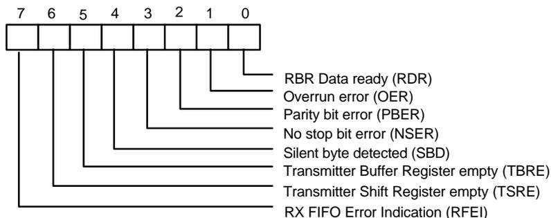
Bit 7: RFEI. In 16450 mode, this bit is always set to a logic 0. In 16550 mode, this bit is set to a logic 1 when there is at least one parity bit error, no stop bit error or silent byte detected in the FIFO. In 16550 mode, this bit is cleared by reading from the USR if there are no remaining errors left in the FIFO.
