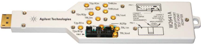
Figure 8: W2641A DisplayPort test point access adaptor.
