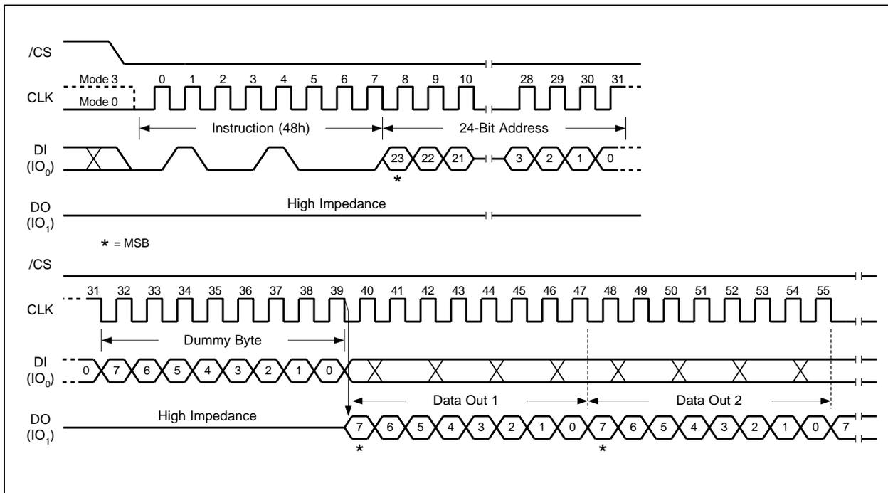
Figure 46. Read Security Registers Instruction (SPI Mode only)
