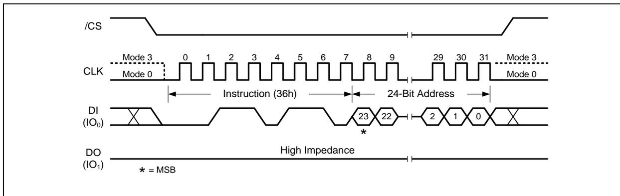
Figure 51a. Individual Block/Sector Lock Instruction (SPI Mode)
