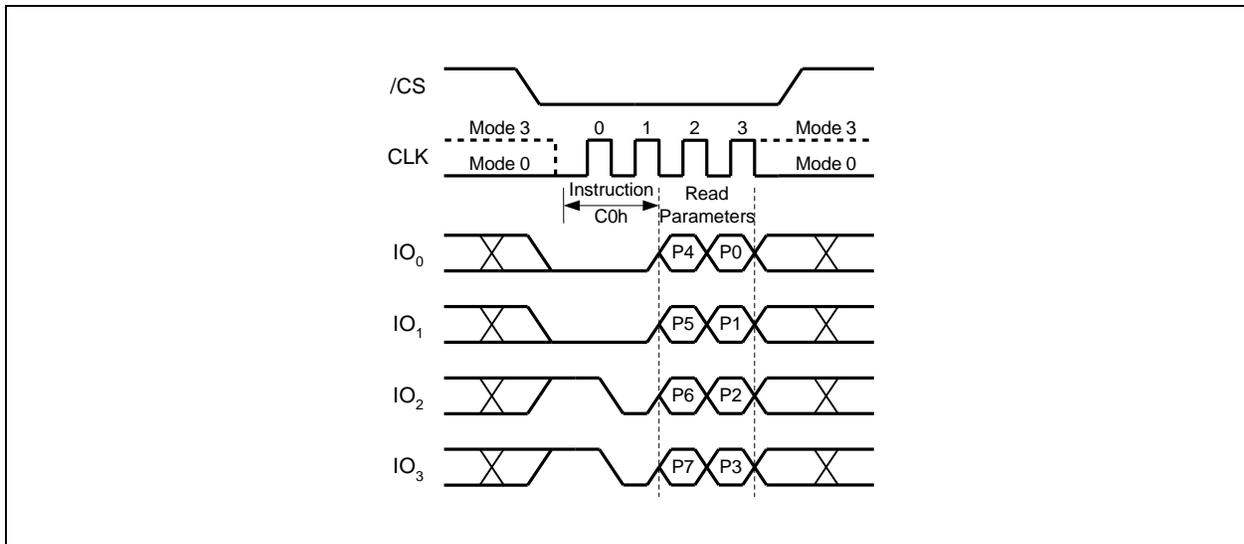
Figure 47. Set Read Parameters Instruction (QPI Mode only)
