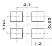
Do not design any conductive path between the pattern
