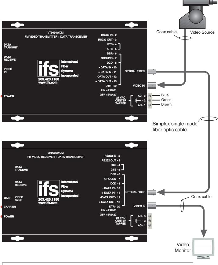
NOTE: WITHOUT PROPER FIBER CONNECTION, LED'S DO NOT INDICATE CORRECT OPERATIONAL STATUS OF THE UNIT.
