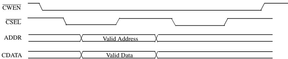
**Figure 3: CPU Interface Functional Read Cycle Timing**
