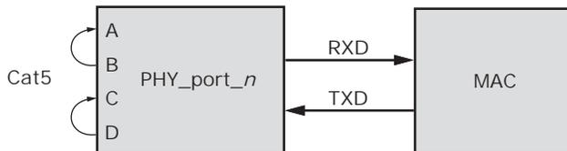
When using the connector loopback testing feature, the device autonegotiation, speed, and duplex configuration is set using device registers 0, 4, and 9.
