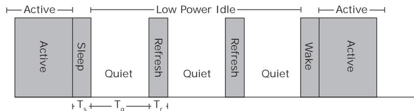
Using LPI, the usage model for the link is to transmit data as fast as possible and then return to a low-power idle state. Energy is saved on the link by cycling between active and low-power idle states. During LPI, power is reduced by turning off unused circuits and using this method, energy use scales with bandwidth utilization. The VSC8514 uses LPI to optimize power dissipation in 100BASE-TX and 1000BASE-T modes of operation.
