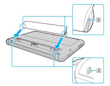
4 Push the battery pack down into the compartment until it clicks into place.
