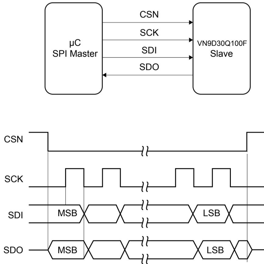
This device can be driven by a micro controller with its SPI peripheral running in the following mode:
