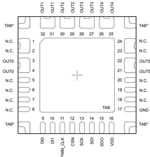
\*: Electrically connected to TAB. Those pins are intended for thermo-mechanical purposes only. They have to be soldered, but must be electrically isolated at PCB level.
