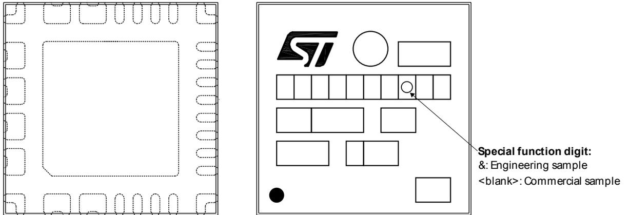
Parts marked as '&' are not yet qualified and therefore not approved for use in production. ST is not responsible for any consequences resulting from such use. In no event will ST be liable for the customer using any of these engineering samples in production. ST's Quality department must be contacted prior to any decision to use these engineering samples to run a qualification activity.
