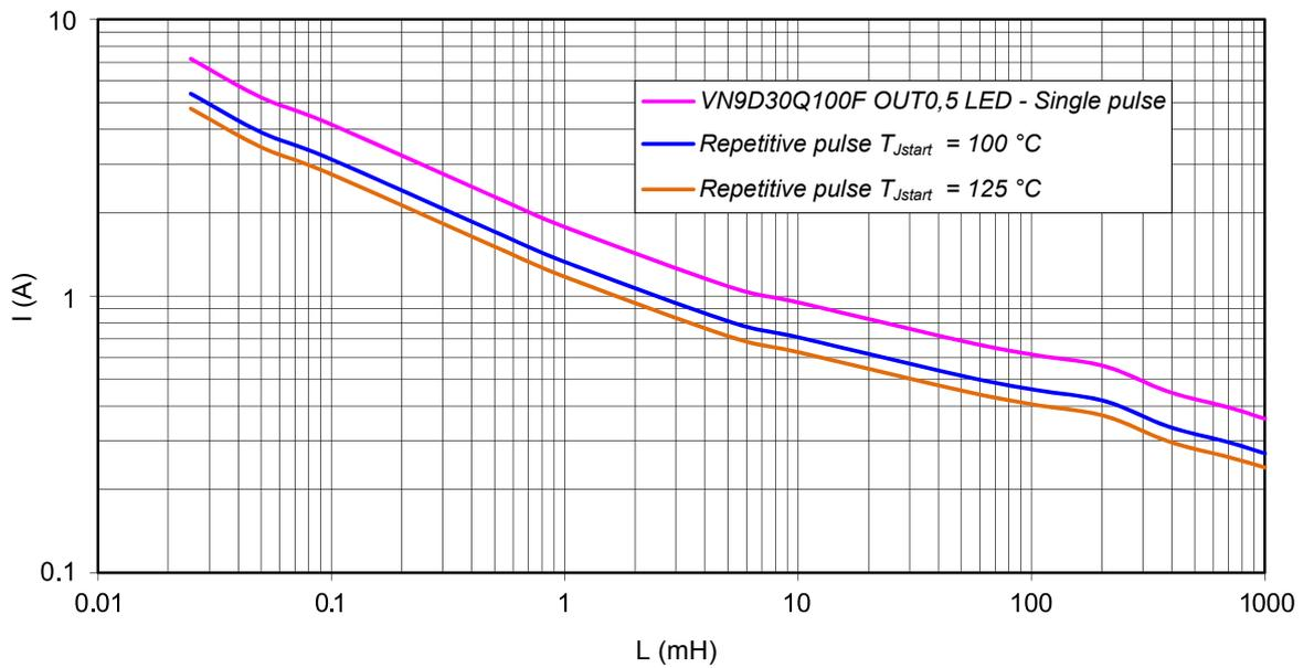
Figure 37. Maximum turn off current versus inductance - Ch1,2,3,4 - Bulb mode
