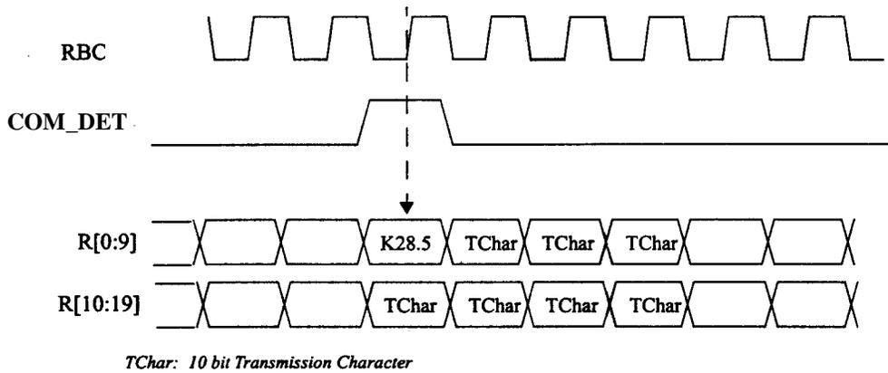
Figure 3. Detection of a Properly Aligned Comma Character
