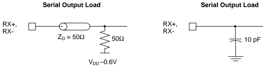
Figure 11. Parametric Test Load Circuit
