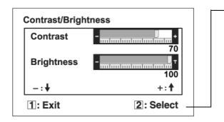
The command line at the bottom of the control screen tells what to do next from this screen. You can toggle between control screens, adjust the selected option, or exit the screen.
