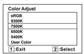
**sRGB-**This is quickly becoming the industry standard for color management, with support being included in many of the latest applications. Enabling this setting allows the LCD display to more accurately display colors the way they were originally intended. Enabling the sRGB setting will cause the Contrast and Brightness adjustments to be disabled.
