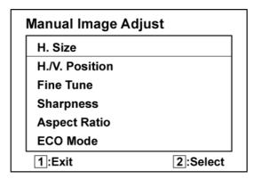
H. Size (Horizontal Size) adjusts the width of the screen image.
