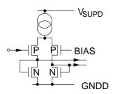
Fig. 4-14: Input pins SAFETY, VPROT, HFLB
