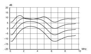
Fig. 2-15: Dynamic peaking frequency response
