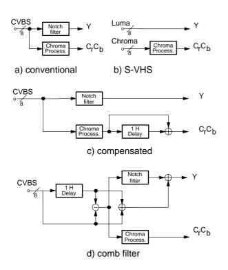
Fig. 2-7: NTSC color decoding options
