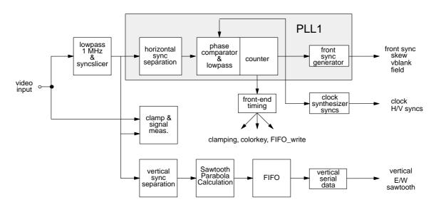
Fig. 2-11: Sync separation block diagram
