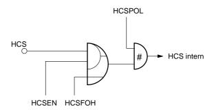
Fig. 2-26: Half Contrast Switch Logic
