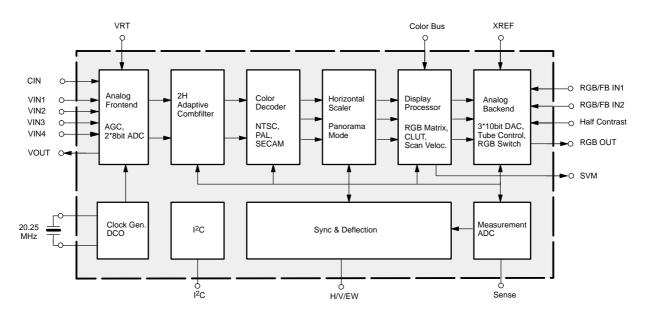
Fig. 1-2: Block diagram of the VDP 3120B
