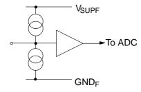
Fig. 4-11: Input pins VIN1-VIN4
