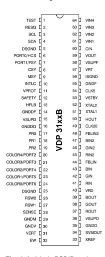
Fig. 4-2: 64-pin PSDIP package
