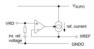
Fig. 4-21: Input pins XREF, VRD
