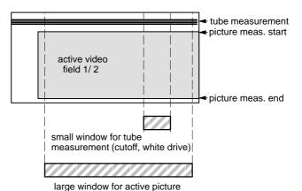
Fig. 2–23: Windows for tube and picture measurements
