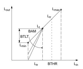
Fig. 2-13: Characteristics of the black level expander
