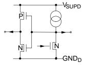
Fig. 4-5: Input/Output pins PR[2:0]
