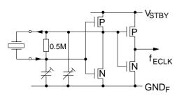
Fig. 4-7: Input/Output pins XTAL1, XTAL2
