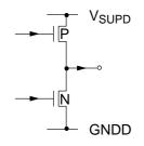
**Fig. 4–13:** Output pins FSY, MSY, CSY, INTLC, PORT[6:0]
