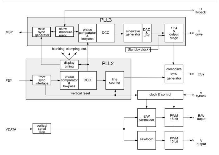
Fig. 2–28: Deflection processing block diagram
