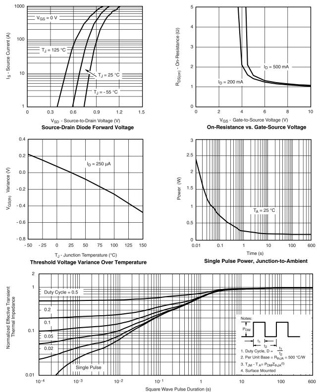
Normalized Thermal Transient Impedance, Junction-to-Ambient
