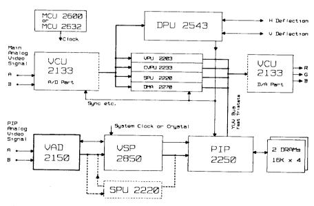
Fig. 1-1: Picture-in-picture block diagram
