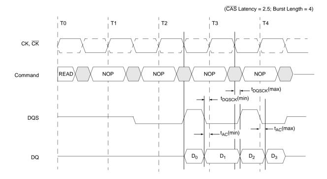
The minimum time during which the output data (DQ) is valid is critical for the receiving device (i.e., a memory controller device). This also applies to the data strobe during the read cycle since it is tightly coupled to the output data. The minimum data output valid time  $(t_{DV})$  and minimum data strobe valid time  $(t_{DQSV})$  are derived from the minimum clock high/low time minus a margin for variation in data access and hold time due to DLL jitter and power supply noise.
