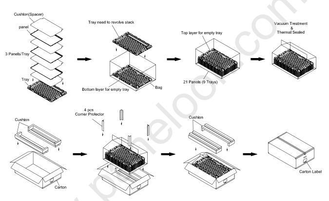
Figure.9-1 packing method
