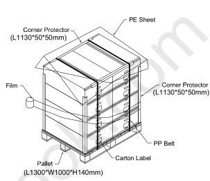
Figure.9-2 packing method
