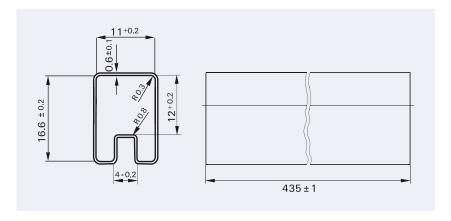
Tube dimensions 25 relays per tube 625 relays per box Our commitment. Your advantage. Telecom-, Signal and RF Relays
