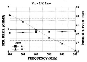
SERIES INPUT IMPEDANCE vs FREQUENCY
