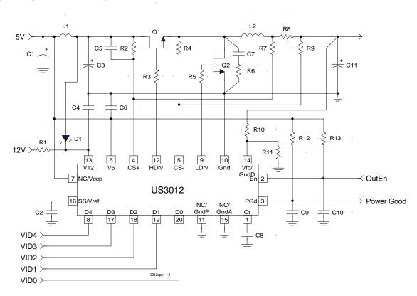
Typical application of US3012/3012A in an on board DC-DC converter providing the Core supply for the Pentium II microprocessor.
